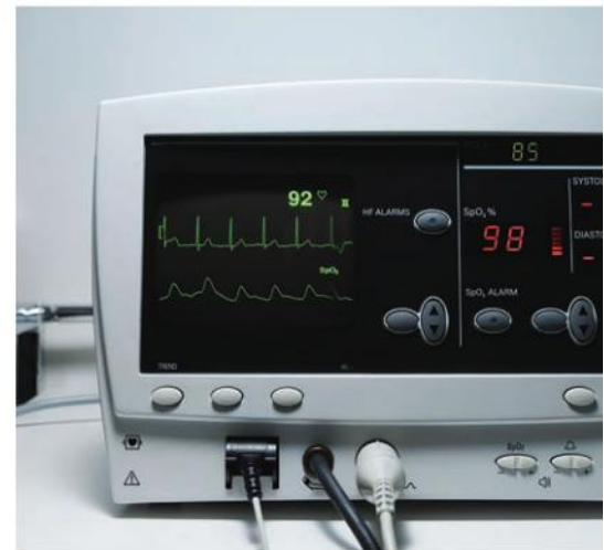
▲ Figure 13 Heart monitor displaying the heart rate, the electrical activity of the heart and the percentage saturation with oxygen of the blood
