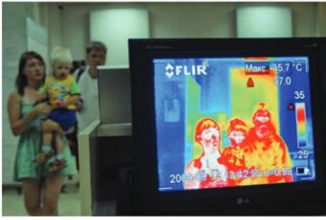
▲ Figure 14 A thermal scanning camera is being used to monitor the skin temperature of passengers arriving at Nizhny Novgorod airport, in Russia. Raised skin temperature can be an indicator of fever from illnesses. Such cameras have been used widely to screen for possible carriers of various possible zoonotic epidemic influenzas such as bird flu and swine flu
