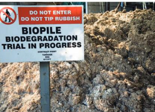
▲ Figure 1 Soil undergoing bioremediation at Fawley Refinery, an oil refinery and chemical plant located in Fawley, Hampshire, UK
