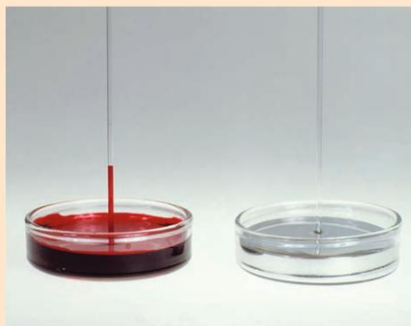
▲ Figure 3 Capillary tubes dipped into water with dye and mercury. Unlike water, there is no adhesion of mercury to the glass nor is there cohesion between mercury atoms, so the mercury does not climb the glass
